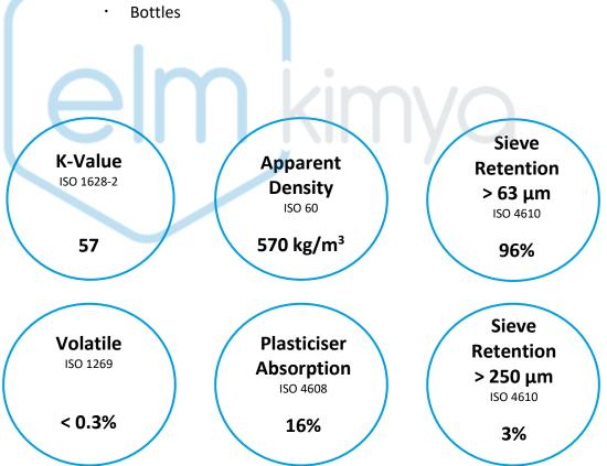
Note: The property data shown above has been obtained from laboratory tests on representative samples of VYNOVA<sup>TM</sup> S5730 polymer. Although the values are typical, they are for guidance only, and must not be used as a basis for specifications.
