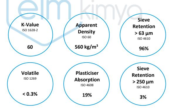
Note: The property data shown above has been obtained from laboratory tests on representative samples of VYNOVA<sup>TM</sup> S5902 polymer. Although the values are typical, they are for guidance only, and must not be used as a basis for specifications.
