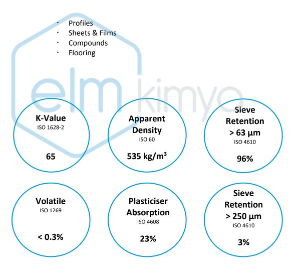
Note: The property data shown above has been obtained from laboratory tests on representative samples of VYNOVA<sup>™</sup> S6502 polymer. Although the values are typical, they are for guidance only, and must not be used as a basis for specifications.
