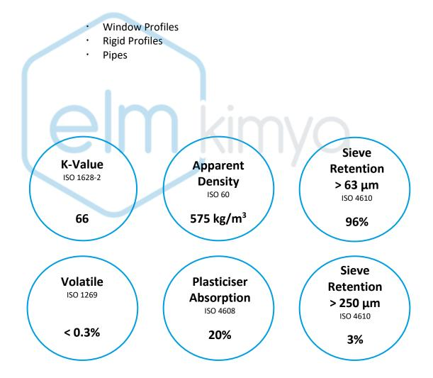
Note: The property data shown above has been obtained from laboratory tests on representative samples of VYNOVA<sup>TM</sup> S6706 polymer. Although the values are typical, they are for guidance only, and must not be used as a basis for specifications.
