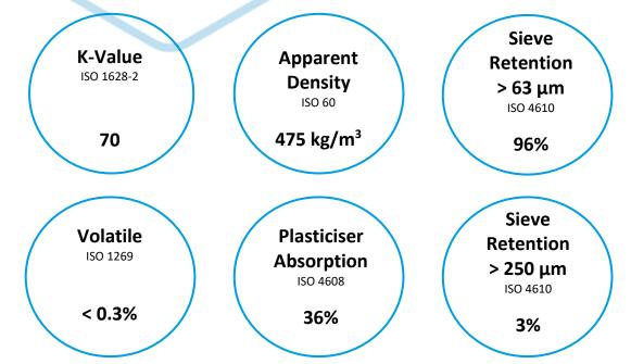
Note: The property data shown above has been obtained from laboratory tests on representative samples of VYNOVA<sup>™</sup> S7000 polymer. Although the values are typical, they are for guidance only, and must not be used as a basis for specifications.
